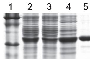
FIG. 1—SDS-PAGE analysis of fractions of aldo-keto reductase 7A2 purification: 10 µg of MW markers (1), 30 µg of proteins from crude (2), flow-through (3), and wash (4) fractions, and 5 µg of purified protein from the elution fraction (5).
