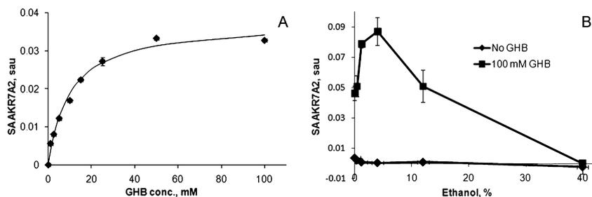
FIG. 3—(A) Michaelis–Menten kinetics of a coupled *aldo-keto reductase* 7A2 (AKR7A2)-*diaphorase-2,6-dichlorophenolindophenol* (DCIP) reaction. Specific activity (SA) units are  $\mu\text{moles DCIP consumed/min per mg protein}$ . At its maximum, the change of absorbance at 600 nm was 0.16/min. (B) AKR7A2-PMS-DCIP coupled reaction with 0%, 0.4%, 1.2%, 4.0%, 12.0% and 40.0% ethanol with and without *Gamma-hydroxybutyrate* (GHB).
